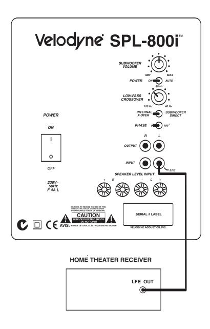
Figure 1. Installation Using LFE Line-Level Inputs
